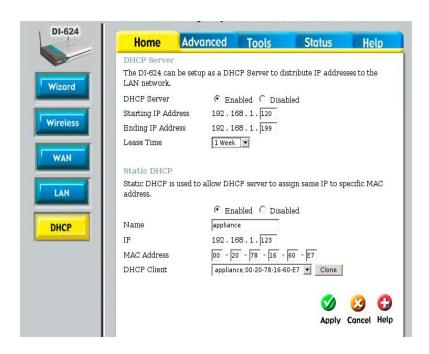
If your router does not support the Static DHCP feature, then you will want to set the IP Address explicitly. Choose a new address value that is not already assigned and is outside of the range of the DHCP server to avoid address conflict. (i.e. does not fall within the Starting and Ending IP Address). Use the new address in the following setup. If you do re-assign the IP address, remember to also set it in the Lorex Monitor using the Lorex Utility (see the manual on how to do this).
